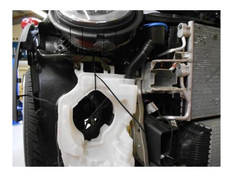
17. Using a flat blade screwdriver or similar remove the 2x clips inside the wheel arch. Using T27 Torx driver undo the one screw. Lift the duct upwards to release it and remove it from the vehicle.
