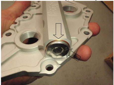
25. Fit the 2x Bonded washers and 2x M22 to AN-10 adapter to the adapter plate.
