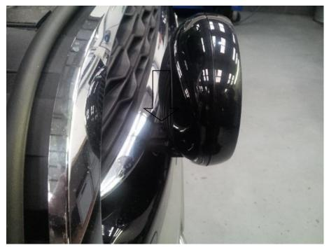
8. Undo the 3x T30 Bolts across the top of the bumper. You will require a second person to carefully pull the bumper forward and clear of the vehicle. Store in a safe place to prevent it from getting damaged while carrying out the rest of the installation.
