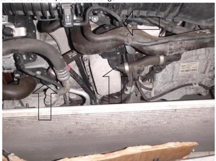
20. Using an E11 Torx socket and suitable ratchet undo the remaining 4 bolts.
