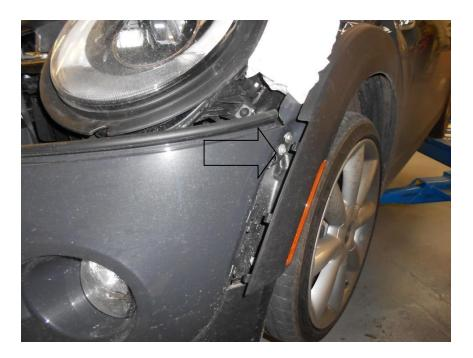
7. If your vehicle is fitted with optional spotlights, use a 3mm Allen key to loosen the horizontal bolt. Tilt the light forward, using a 2mm Allen key undo the bolt and remove
