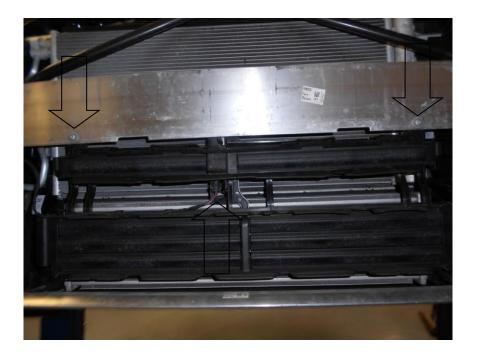
11. Undo 3x T30 Torx screws and remove the front brace.
