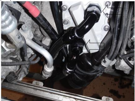
30. Feed the other end of the 2x oil lines between through the gap shown below on the near-side of the car. Use the silicone sleeve and cable ties provided to protect the two oil lines in the area that they pass the intercooler mounting bracket.
