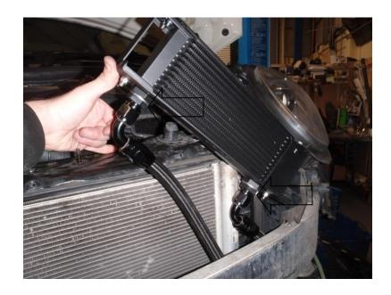
37. Place the oil cooler and bracket in position on the crashbar. Refit the OEM bolt to the top mounting tab. Ensure that your pilot holes are visible in the base plate of the bracket.
