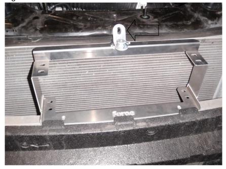
32. Using a scriber or marker pen mark the positions of the two holes in the base plate of the bracket on the crash bar.
