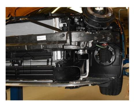
10. If fitted to your vehicle, unclip the wiring and using a T30 Torx driver undo the 2x bolts and remove the active air ducting. This part will not be refitted to the vehicle when the installation is complete.
