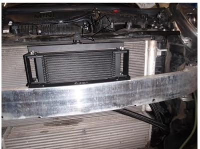
38. Using a 8mm Nut driver on a battery drill install the 2x 5.5x25mm Tech-screws into the crash bar. These are self-tapping screws. Over tightening these screws runs the risk of pulling the thread out of the crash bar.
