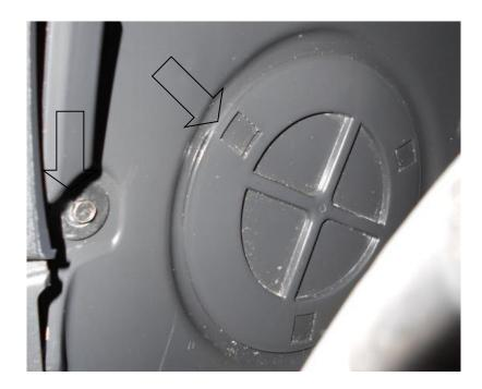
5. Using a 10mm socket, extension bar and suitable ratchet undo 2x 10mm nuts. Unclip the scoop at the airbox and remove the intake scoop.
