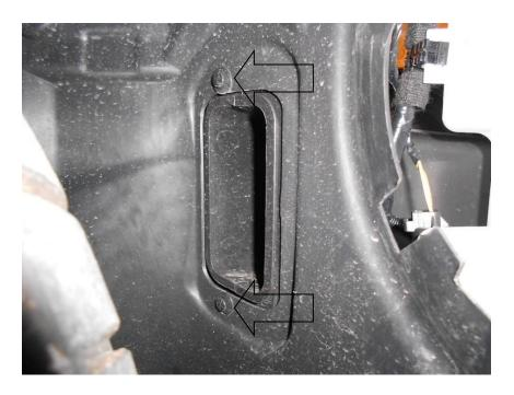
15. Using T27 Torx driver undo 1x screw and unplug the temperature sensor. Lift the duct upwards to release it and remove it from the vehicle.
